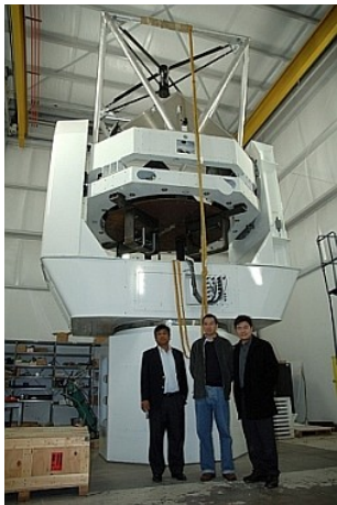
2.4m telescope of the same specification that will be installed in NARIT's observatory on Doi Inthanon
